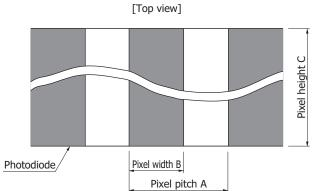
S11637 series: A=12.5  $\mu$ m, B=8.5  $\mu$ m, C=500  $\mu$ m S12198 series: A=25  $\mu$ m, B=20  $\mu$ m, C=500  $\mu$ m
