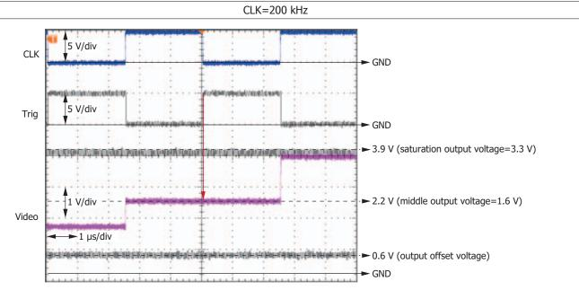
Note: On the waveform of the middle output voltage shown above, in order to make it easier to identify the output of each pixel, the light was input so that the outputs of the adjacent pixels appeared in a step form.
