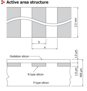
S3901 series:  $a=50 \ \mu m$ ,  $b=45 \ \mu m$ S3904 series:  $a=25 \ \mu m$ ,  $b=20 \ \mu m$
