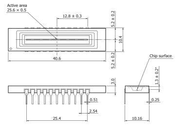
\* Optical distance from the outer surface of the quartz window to the chip surface
