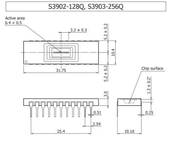
\* Optical distance from the outer surface of the quartz window to the chip surface
