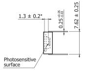
\* Distance from upper surface of window to photosensitive surface
