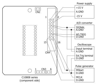
Note: Mount the connector at CN4 on the component side. Install the CMOS linear image sensor into position while aligning pin no. 1 with the index mark (pin no. 1) on the back side of the C10808 series.
