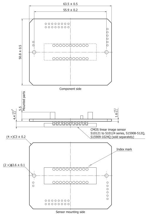
\* When CMOS linear image sensor pins are fully inserted into board.
