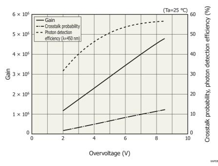
MPPC characteristics vary with the operating voltage. Although increasing the operating voltage improves the photon detection efficiency and time resolution, it also increases the dark count and crosstalk at the same time, so an optimum operating voltage must be selected to match the application.
