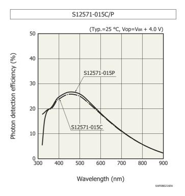
Photon detection efficiency does not include crosstalk or afterpulses.
