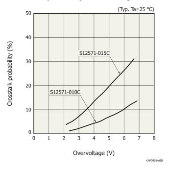
Because the high-speed, wide dynamic range MPPC has a small pixel capacitance, the gain is smaller than the MPPC for general measurement. The gain and photon detection efficiency are increased by applying the higher operating voltage. Please use it with the appropriate operating voltage because the crosstalk increases at the same time.
